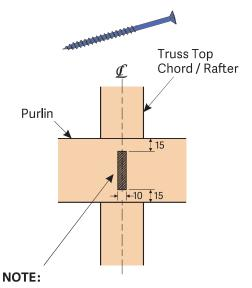
Locate fixings within the shaded area. Care to be taken to avoid over tightening of Screws.
