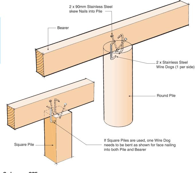
Code:OPFPacked:20 x Stainless Steel Wire Dog Staples<br/>20 x Stainless Steel Nails 90mm x 4 dia.
