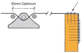
$\begin{array}{l} 0.91 mm \times 53 mm \ G300 \ Z275 \ GALVANISED \ STEEL \\ 0.9 mm \times 53 mm \ STAINLESS \ STEEL \ 304-2B \end{array}$
