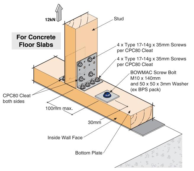
Code:SBPMaterial:CPC80 1.55mm G300 Z275 Galvanised SteelPacked:2 x CPC80 Cleats<br/>16 x Type 17-14g x 35mm Hex Head Galvanised Screws
