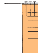
3 nails top edge, 8 nails vertical face (not in same line)
