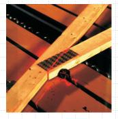
Precision location of the connector plate on the joint.
