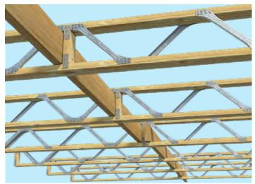
Improved rigidity & stiffness, reduced bounce, minimal movement, firm under foot
